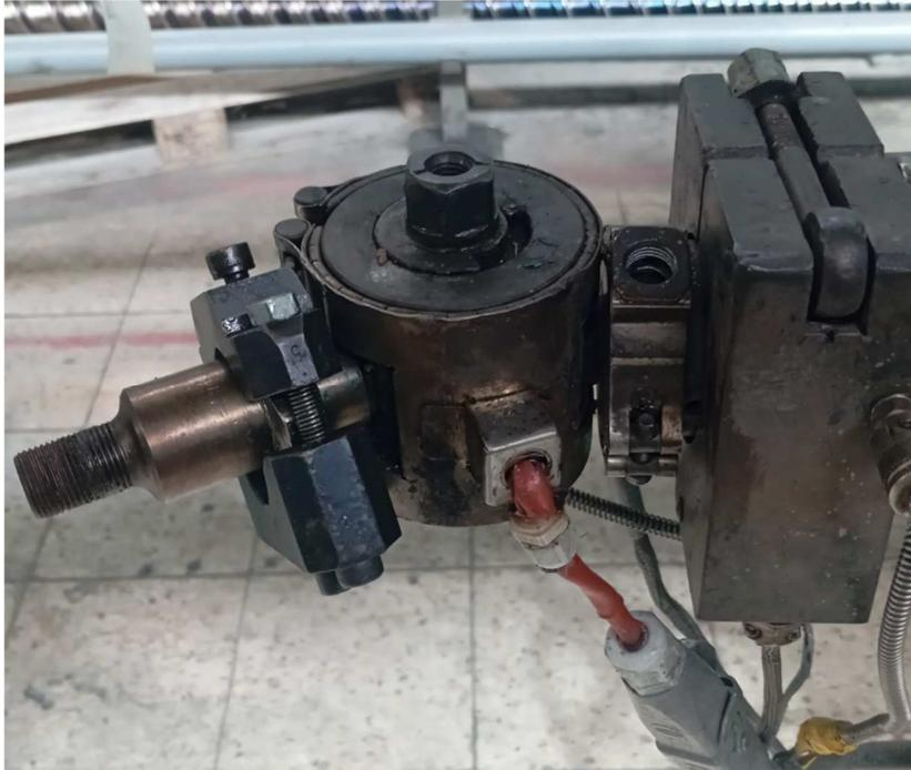
Above distributor should be connected to the extrusion head somewhere as seen on below picture:
